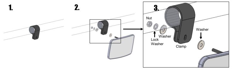
Open the clamp with two hands and snap around roll cage. Be careful when releasing the clamp to avoid pinching fingers. The flange should face toward viewer. Loosely attach Mirror with hardware shown above. The washers should go on either side of the plastic clamp. The lock washer goes between the washer and nut. You will tighten completely after adjustments.
