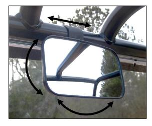
Adjust the mirror along the roll cage and angle as needed. Fully tighten locknut.
