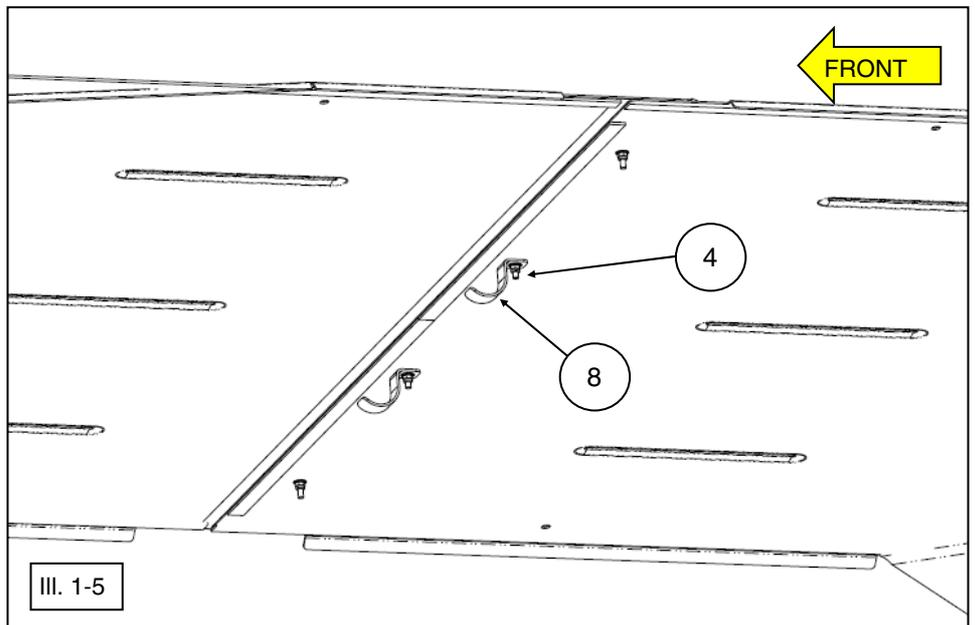
5. Place roof assembly on the top of the vehicle cab frame.
