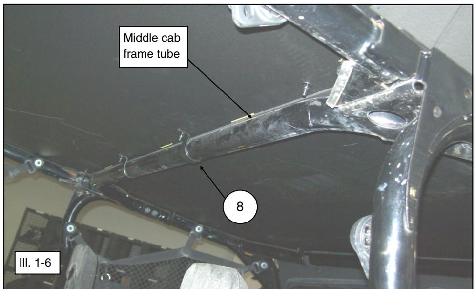
6. Align the center clamps (item #8) onto the middle cab frame tube, so that these can be fit onto the tube. (See illustration 1-6).
