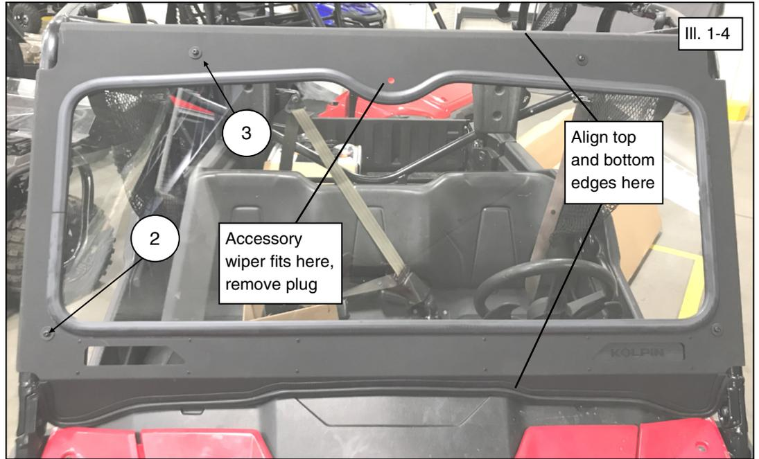
6. Center the windshield onto the cab frame and then from rear windshield surface, place clamps (item #5) around cab frame tubes and fasten with M6 locknuts (item #4) as shown. (See illustrations 1-5 and 1-6).
