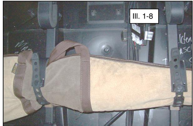
**WARNING:** Make sure the gun (or bow) does not extend below or outside the vehicle frame as severe damage could result to your firearm (or bow) inside if obstructions are encountered.
