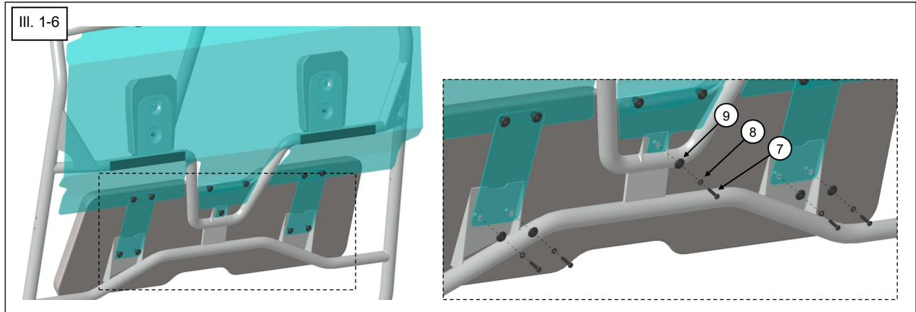
11. On both Headrests, position the Nylon Spacer [Item 11] between the Threaded Coupling Nut [Item 13] and the Upper Panel. Then insert the Domed Shoulder Washer [Item 9], Lock Washer [Item 8], and Button Head Screw - M6 x 26mm [Item 7]. See Illustration 1-7.
