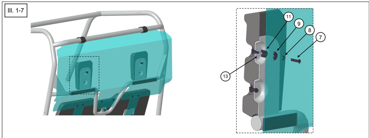
12. Assure the Windshield is aligned evenly before tightening hardware.
