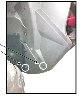
Over-tightening any and/or all screws will cause cracks around mounting holes which is not covered by any warranty.
