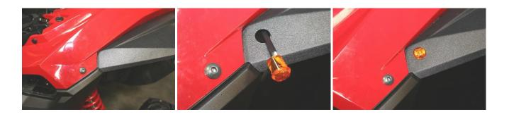
6. Mount Billet Turn Lever – Run the billet handle wire from the ATS control Module to the steering wheel, remove the screw that holds the steering wheel tilt lever, discard the hardware removed, install the lever bolt through the removed bolt hole, make sure to put the new supplied bushing in the center and secure with the included nut. Line switch housing up and tighten mounting nut. Secure wire harness with included cable ties.
