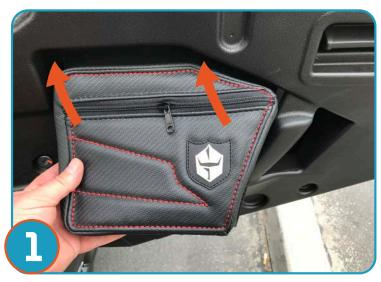
Remove velcro® strip on back of door pad and place door bag into door cavity inserting top backing at an angle. Door bag will then fall into place. Press firmly on bag to adhere velcro strip to door panel.
