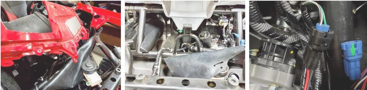
2. Next to the Power Steering unit is a blue connector, un-plug the blue connector from the holder by lifting on the small center tab. Plug in the adapter, attach the device to be powered, all devices installed should have there own in-line fuse
