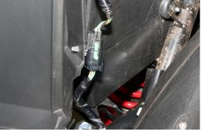
3. Unplug that connector and plug this adapter inline. If you have our Turn Signal System installed, plugging this adapter inline after will include the signals, before will only give brake out on the Green and Yellow wires.
