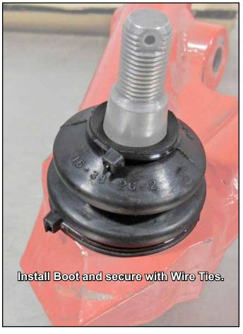
Torque to factory setting when resecuring to Knuckle.
