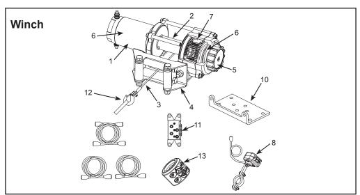
**Motor (1):** 1.2 HP 12V DC motor provides power to the planetary gear mechanism.
