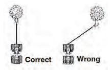
Short pulls from an angle can be used to straighten the vehicle. Long pulls should be done with the wire rope at a  $90^\circ$  angle to the winch/vehicle.
